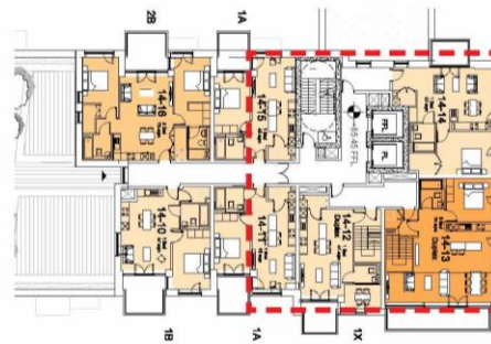
Outline of footprint achieving 3:1 slenderness ratio overlaid over current plan - this footprint would only allow for 3 apartments per floor.
